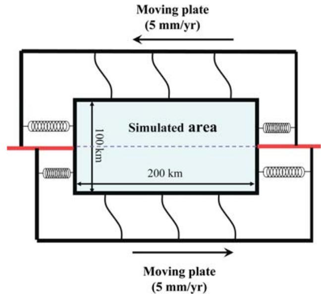
**Figure 6.** A schematic diagram illustrating the generalized boundary conditions corresponding to a constant plate motion far from the simulated model region.
