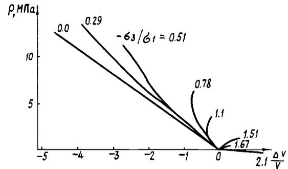
Fig. 1. Average pressure versus cubic strain of Westerly granite sample under load.
