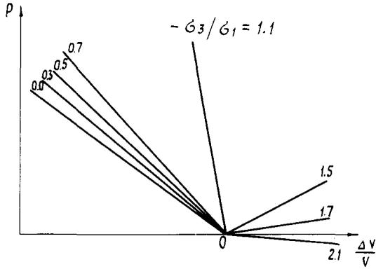
Fig. 2. Simulated average pressure versus cubic strain dependences.
