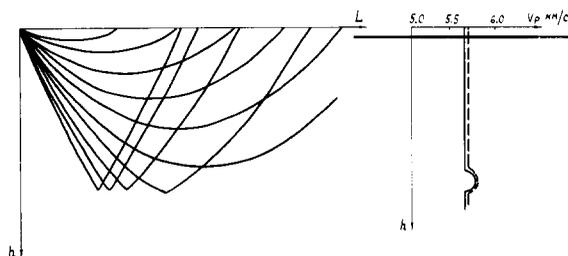
Fig. 3. Velocity distribution and ray paths (variant one): — — — horizontally propagating waves; ——— vertically propagating waves.
