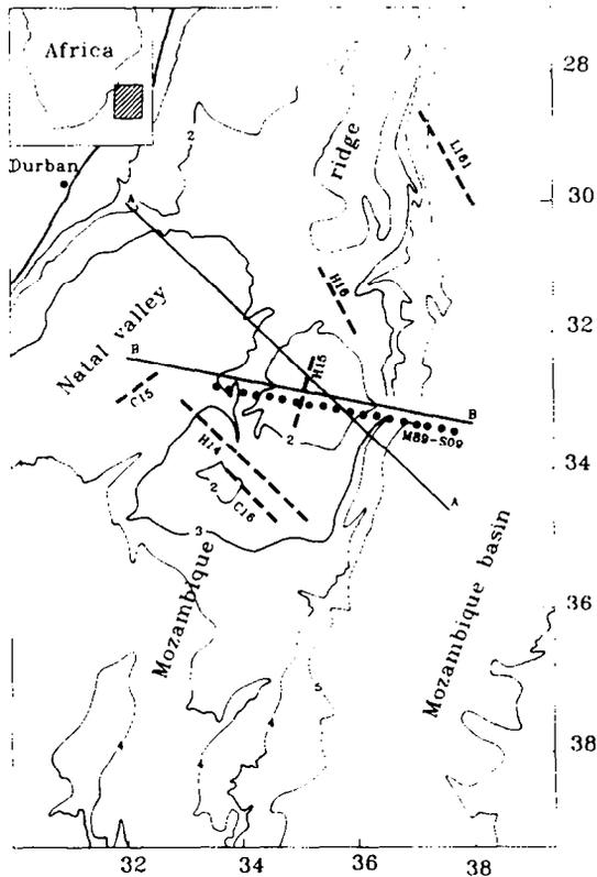
Fig. 1. Bathymetry of the investigated area after Dingle et al. (1987); contour interval 1 km. Solid line *A-A* = profile investigated by Maia et al. (1990) for the direct geoid modelling (Fig. 2). Dotted line = continuous seismic reflection profile M89-S09 (Fig. 3). Dashed lines = refraction profiles, depth of the boundaries from which were projected on the investigated cross-section *B-B* (Fig. 4). Inset shows the regional setting.
