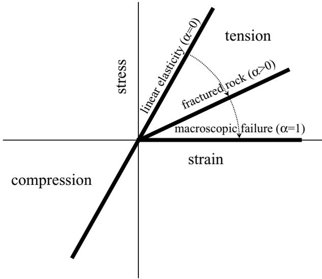
**Figure 4.** Schematic change of the stress–strain with damage. Bilinear behaviour incorporated in the non-linear damage model provides significantly improved fitting to the experimental data (grey and red lines in Fig. 3).
