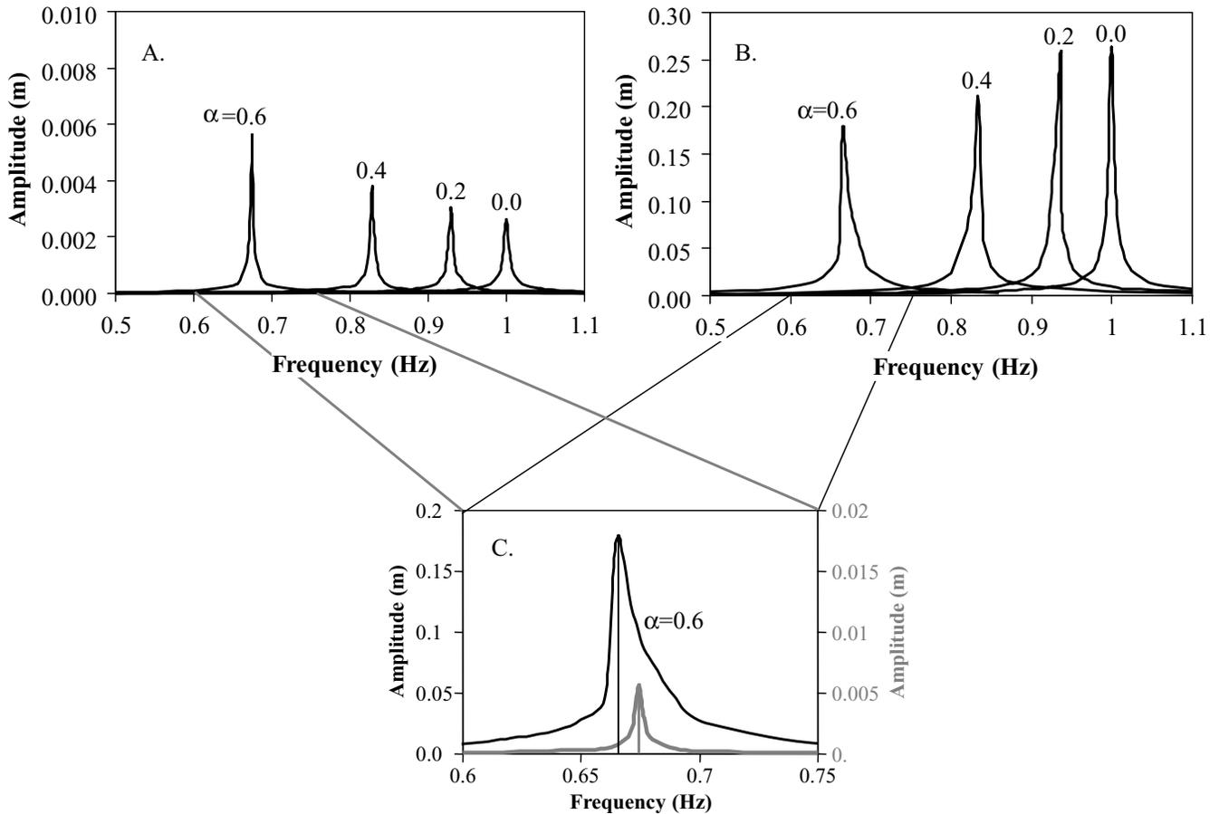
**Figure 8.** Simulated resonance curves for the material damage ranging from  $\alpha = 0$  to 0.6 with 100 Pa (a) and 10 000 Pa (b) periodic forcing. Note that the amplitude scale differs by factor of 50, whereas the forcing is increased by factor of 100. (c) A zoom in view of the small frequency range for the simulation with  $\alpha = 0.6$ . Black line represents the high forcing case, whereas grey line and grey scale on the right corresponds to the small forcing.
