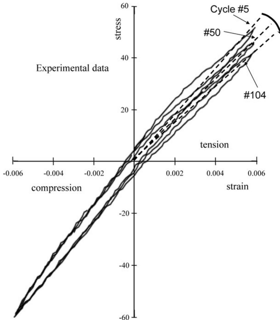
**Figure 1.** Results of strain-controlled uniaxial tension–compression tests on a composite, prepared using lightly cross-linked poly-methyl methacrylate filled with alumina trihydrate (Basaran & Nie 2004). Stress–strain cycles no. 5, 50 and 104 demonstrate gradual decrease in the elastic modulus under tension, whereas the compressional part of the loop remains almost the same.
