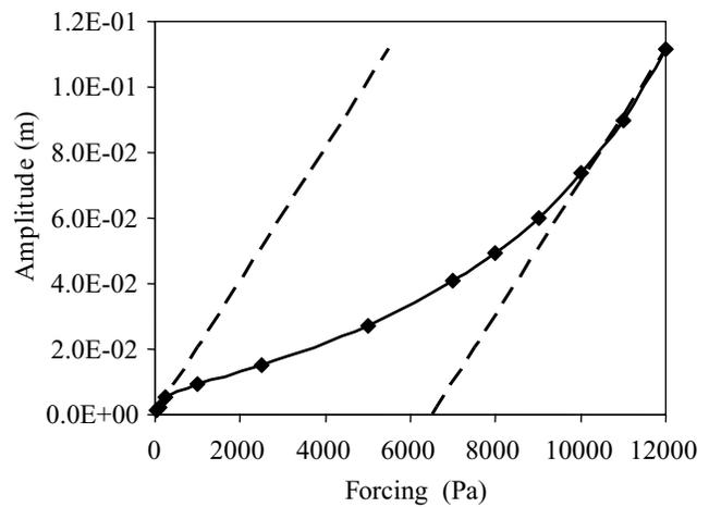
**Figure 7.** Simulated resonance amplitude for different forcing. Dashed lines correspond to the amplitude–forcing relation expected for a linear system with constant quality factor.
