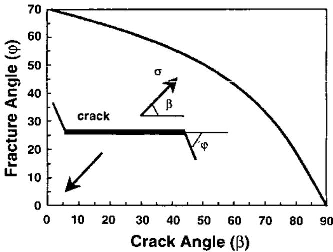
Figure 4. Theoretically predicted and experimentally confirmed relation (Erdogan and Sih<sup>54</sup>) between crack angle  $\beta$  and fracture angle  $\phi$  [equation 16]
