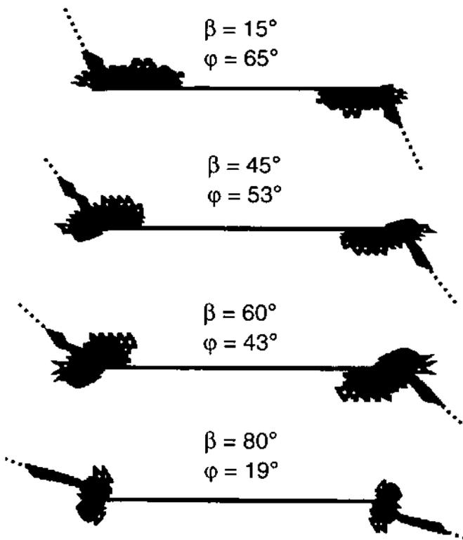
Figure 5. Geometry of the damage zones around the narrow pre-existing fracture subjected to out-of plane load with crack angle  $\beta=15^\circ, 45^\circ, 60^\circ,$  and  $80^\circ$ . Propagation path of highly destroyed zone perfectly fits the theoretically predicted direction (dotted lines)
