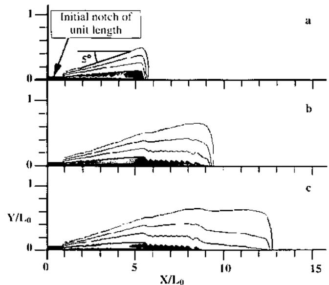
Figure 3. The process zone around the crack has the same geometry until the dynamic weakening is negligible (a). The size of the process zone increases much more slowly when the dynamic weakening becomes important (b), and even decreases at the crack acceleration stage (c)
