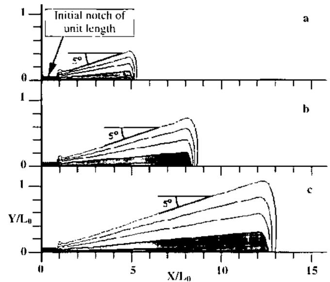
Figure 2. The process zone for three different stages of quasi-static crack growth has self-similar geometry with a constant  $\sim 5^\circ$  slope of the outer boundary. Here and in Figure 3 the step between contour levels is equal 0.1
