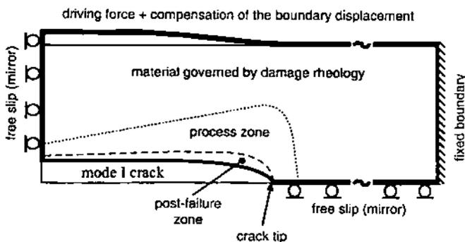
Figure 1. The problem set up for numerical simulation of crack propagation. The variable force vector,  $F_i$ , applied to each node at the top boundary, corresponds to the constant traction force,  $F_d$ , applied infinitely far from the simulated region
