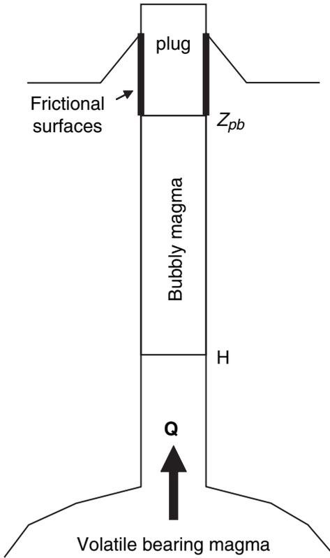
**Fig. 3.** Schematic diagram of the discussed system. The magma at the source contains volatiles, it flows upward in the conduit and from depth  $H$  the magma vesiculates. The plug partially blocks the flow, according to the pressurization processes and friction along plug walls — see text.
