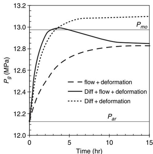
**Fig. 9.** Pressure evolution by diffusion (upper curve), magma flow (lower curve) and their coupled solution (middle curve with maximum).
