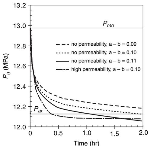
Fig. 6. Depressurization due to plug motion and permeability — see text.
