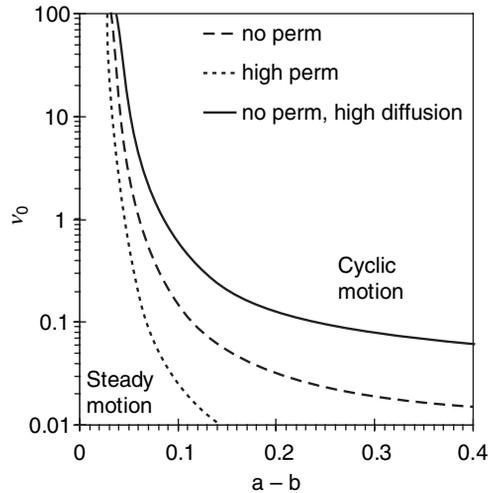
**Fig. 5.** Steady-state solution distinguishes between steady-state extrusion and cyclic motion for a given values of  $(a - b)$  and  $v_0$ .
