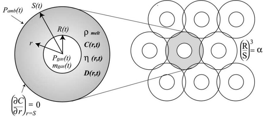
Fig. 1. The physical model. The magma is regarded as a pack of spherical cells, each composed of a gas bubble with radius  $R$  centered in a spherical melt shell with outer radius  $S$ . The cells are arranged in a 3-D lattice with some overlap, so that gas volume fraction is  $\alpha = (R/S)^3$ . (Modified after Proussevitch et al., 1993).
