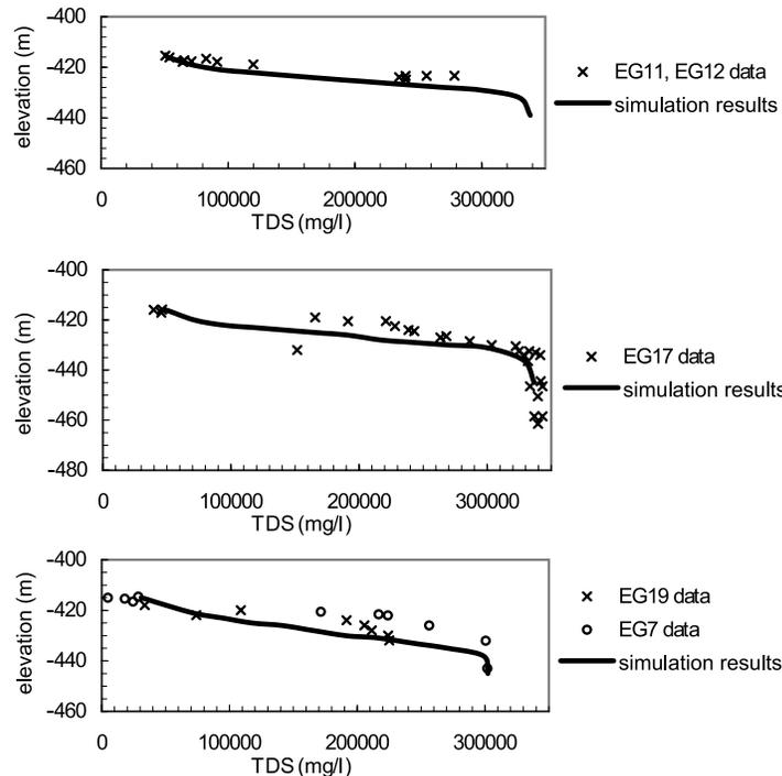
**Figure 12.** Comparison between simulation results of Figure 9 and field data, showing correspondence between the salinity in the field data and the concentration calculated from the simulation (data from Kiro [2006]).
