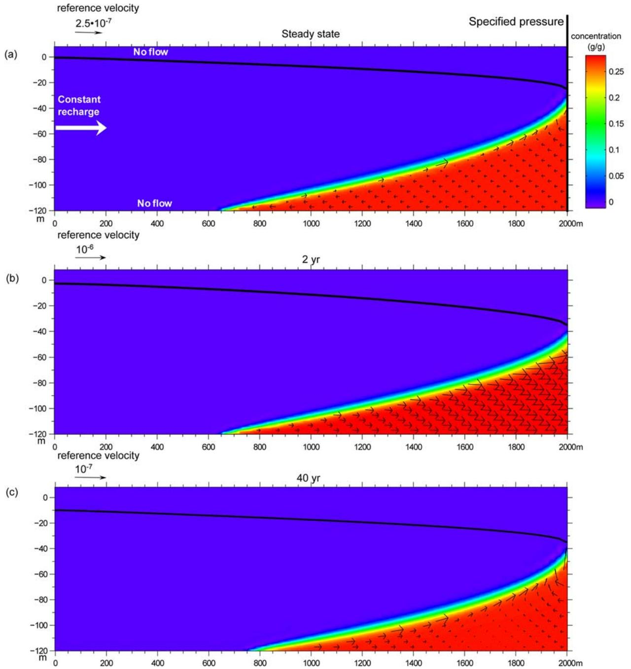
**Figure 4.** Saline water flow after an instantaneous lake level drop; only the velocity of the saline water is given. The parameter values of the presented results are those of the base simulation (Table 2). The steady state conditions are (a) the initial conditions; (b) after the lake level drops the saline water flow is in the direction of the lake; and (c) after a period of time the saline water circulation reestablishes.
