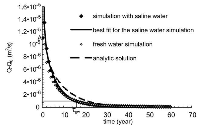
**Figure 3.** Change in the discharge to the Dead Sea ( $Q - Q_0$ ) after an instantaneous level drop: analytic solution (first 1000 terms); fresh water simulation with parameters of the base simulation (Table 2); simulation including a transition zone (Table 2) and its best fit for the parameters  $A$  and  $\tau_{gw}$ . The characteristic time is approximately the time in which the discharge decayed to  $1/\exp(\pi^2/4)$  of its initial value ( $A$ ).
