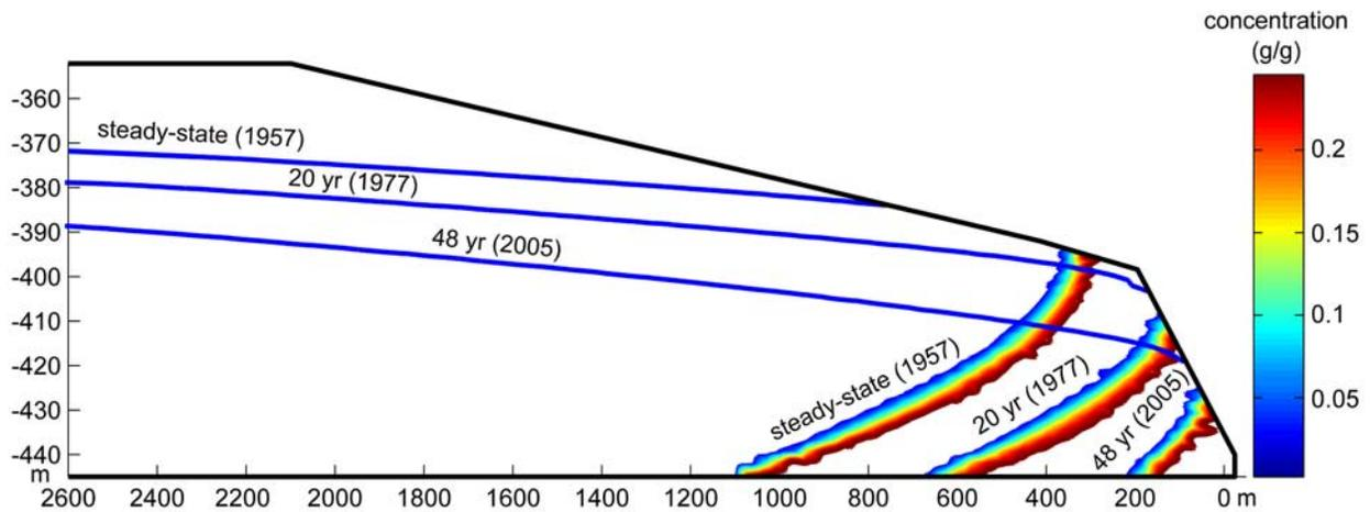
**Figure 11.** Simulation results with a relatively large hydraulic gradient (Table 4;  $k = 1.3 \times 10^{-11} \text{ m}^2$ ;  $Q_0 = 0.06 \text{ kg s}^{-1}$ ). The hydraulic gradient increases considerably, and the transition zone moves relatively fast and is always in equilibrium with the water table.
