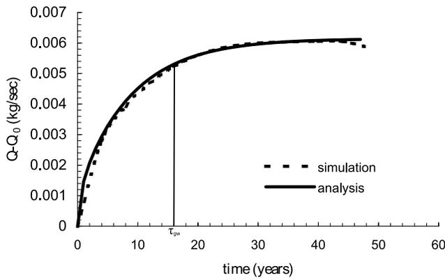
**Figure 7.** Change in the discharge versus time when the lake level drops continuously. The parameter values of the presented results are those of the base simulation (Table 2) with  $R = 0.5 \text{ m a}^{-1}$ .
