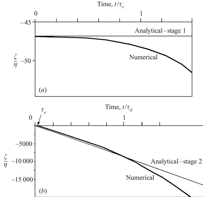
FIGURE 5. Bulk viscosity vs. time. The calculation uses the parameters listed in table 1. (a) During stage 1, at  $t < \tau_v$ , the bulk viscosity is negative and deviates by less than 10% from the analytically calculated value (3.4). Time is scaled to  $\tau_v$  and bulk viscosity is scaled to the melt shear viscosity. (b) During stage 2, when  $\tau_v < t < \tau_d$ , the bulk viscosity is negative and the numerical solution follows the linear approximation of the analytical solution (3.6).
