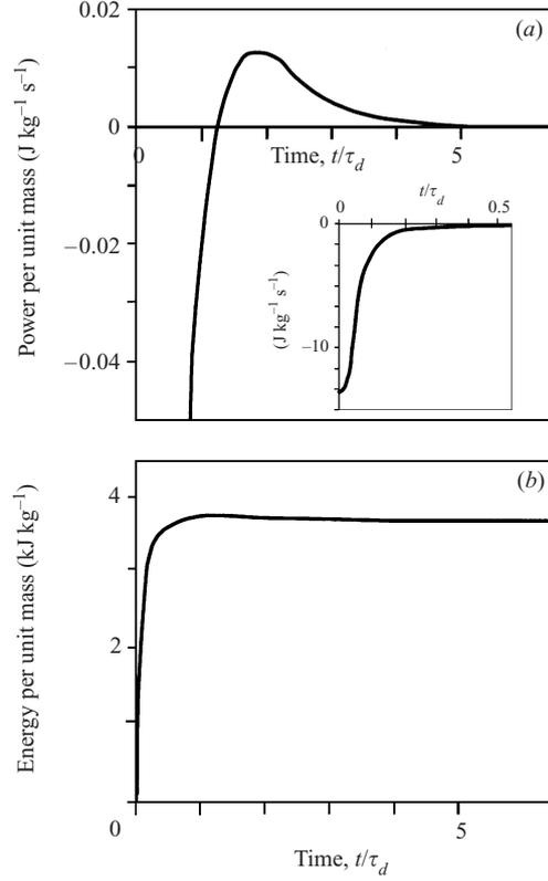
FIGURE 7. (a) Mechanical power of the expanding cell and (b) the energy of expansion, over time.
