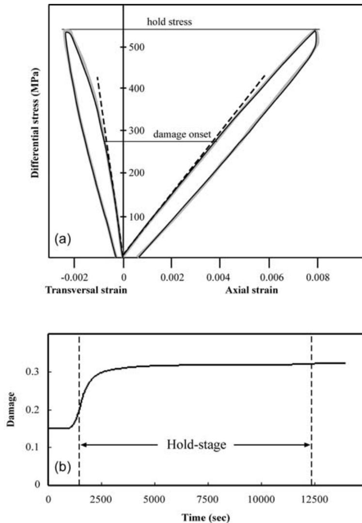
**Figure 4.** (a) Measured stress–strain curves, axial and transversal, for sample 109 (grey line) compared to the model prediction (black line). Dashed line represents the solution assuming linear elasticity. The values of the hold stress and onset of damage are shown by thin black lines. (b) Simulated evolution of damage ( $\alpha$ ) during the experiment. See Table 2 for model coefficients.
