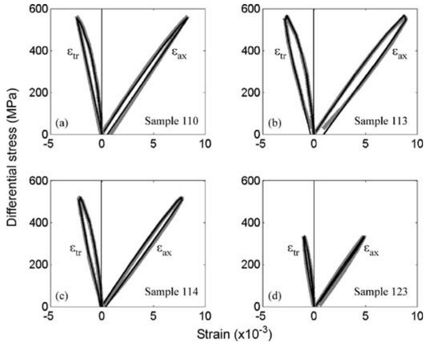
**Figure 7.** Measured stress–strain curves (grey line), axial and transversal, for samples that were loaded and then analysed for crack density [samples: 110 (a), 113 (b), 114 (c), 123 (d)] compared with the calculated curve (black line). For model coefficients see Table 2.
