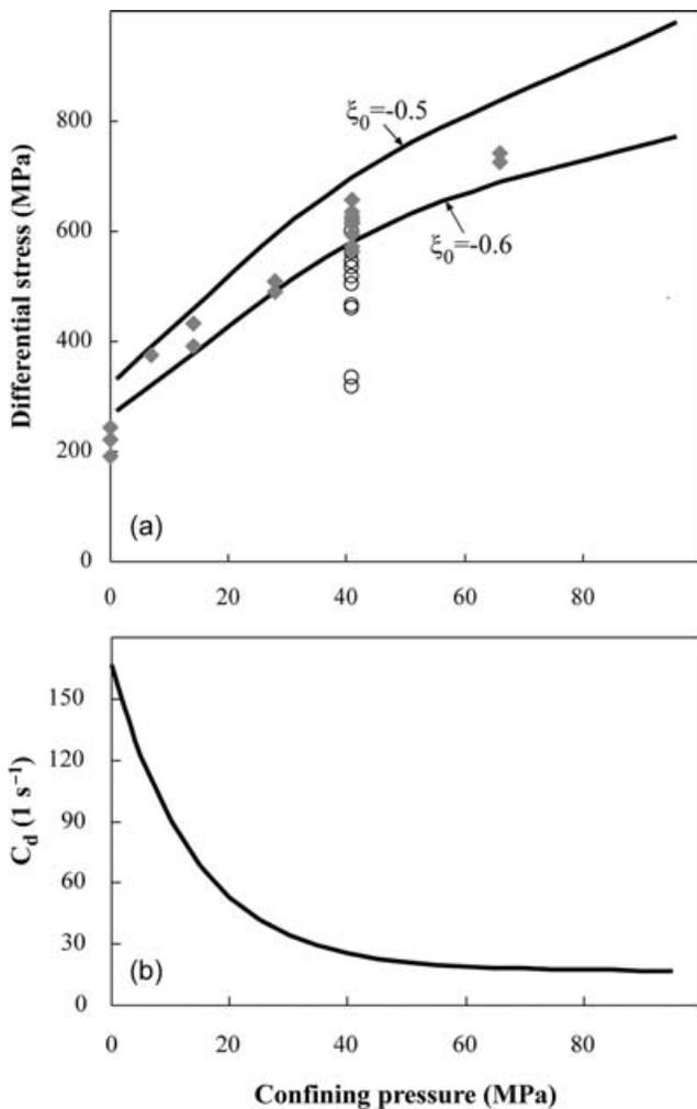
**Figure 9.** (a) The measured failure stress versus confining pressure (grey diamonds) compared with calculated failure curves for  $\xi_0 = -0.5$  and  $\xi_0 = -0.6$  ( $C_v = 1.5 \times 10^{-5} \text{ MPa}^{-1}$ ). The stress at which the load-hold experiments were held (without failure of the sample) is shown by empty black circles. (b) The damage rate coefficient,  $C_d$ , versus confining pressure used for calculating the curves for the Mount Scott granite shown in (a).
