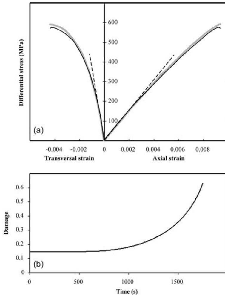
**Figure 6.** (a) Measured stress–strain curves, axial and transversal, for sample 103 (grey line) compared to the model prediction (black line). Dashed line represents the solution for linear elasticity. (b) Simulated evolution of damage ( $\alpha$ ) during the experiment. Note the different damage evolution here compared to the load hold tests 109 (Fig. 4) and 115 (Fig. 5).
