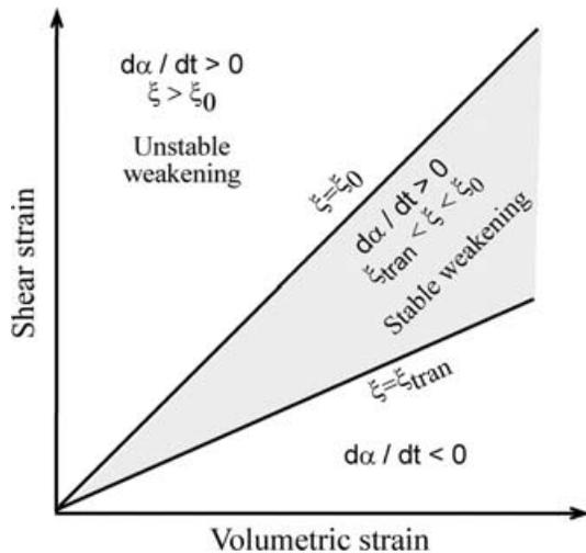
**Figure 3.** Schematic diagram of the states of strain associated with unstable and stable material weakening, and healing in our model. Unstable weakening occurs when  $\xi \geq \xi_0$ ; stable weakening occurs when  $\xi_{\text{tran}} \leq \xi < \xi_0$ ; and healing occurs when  $\xi < \xi_{\text{tran}}$ .
