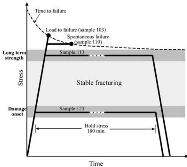
**Figure 1.** Schematic diagram of the loading and types of experiments. Dark grey areas represent some variability in the onset of damage and the long term strength as deduced from the experiments. Light grey area represents the region where the damage evolution has steady-state solution, and dashed line represents the time-to-failure curve. The sample numbers denote experiments performed at different conditions.
