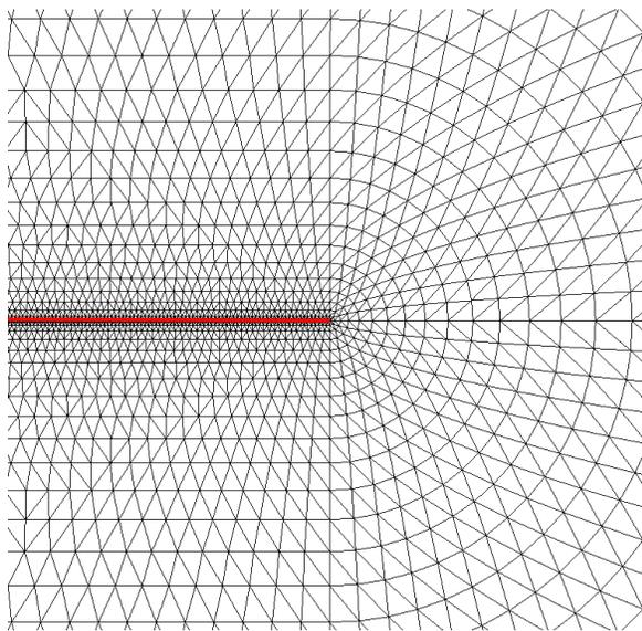
**Figure 2.** Mesh geometry around the tip of a preexisting narrow damage zone colored in red. The mesh consists of triangle elements with gradually increasing size away from the crack tip. The width of the damage zone (smallest element size) is one thousandth of the damage zone length.
