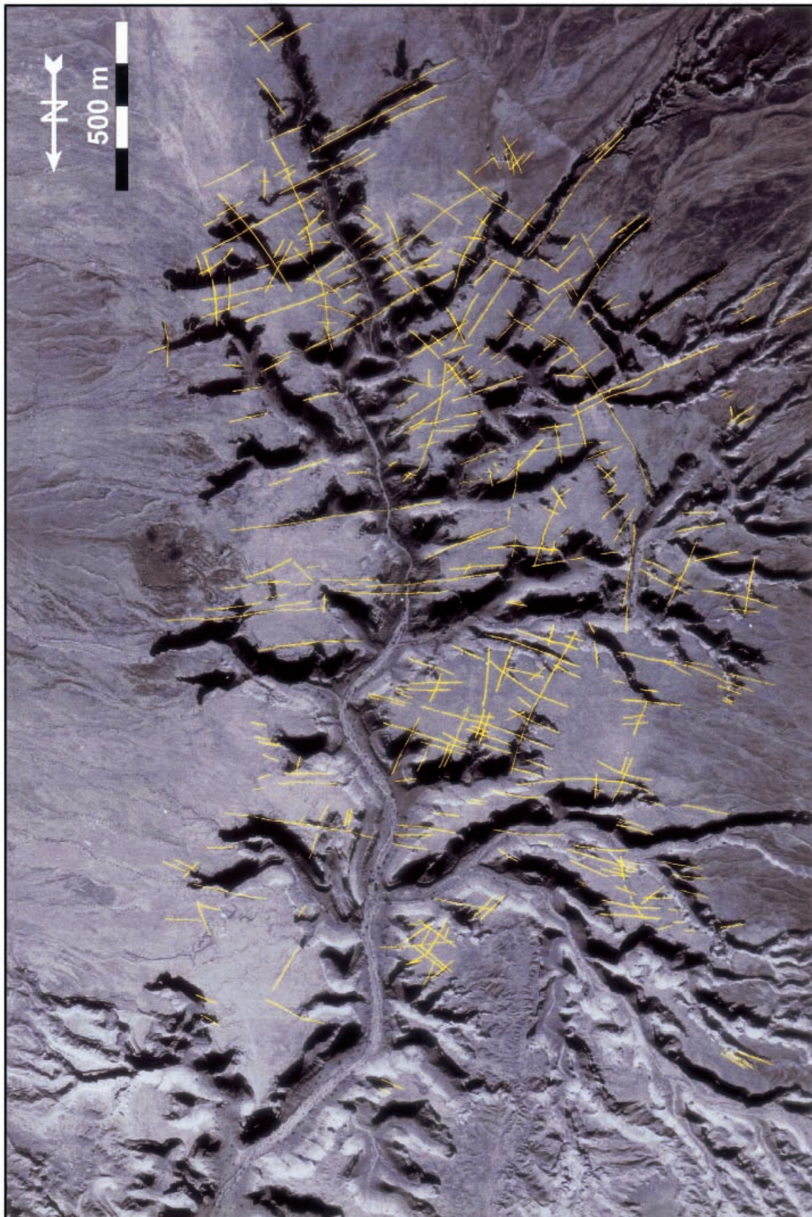
Fig. 4 Map of fracture traces (yellow lines). Background aerial photograph by the Survey of Israel.
