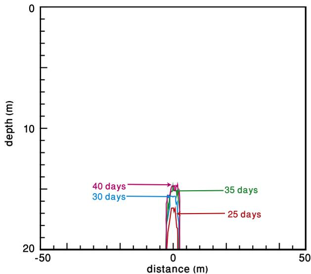
**Fig. 4.** Cavity configuration evolution for a damage controlled simulation of deformation caused by a 10 m-wide underlying cavity. These results are similar to field observation in the alluvial fans (Fig. 2b).
