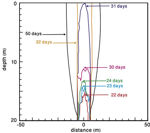
**Fig. 6.** Cavity configuration evolution for a mixed damage and visco-elastic simulation of deformation caused by a 10 m-wide underlying cavity. These results are similar to field observations in the mud-flat (Fig. 2a).
