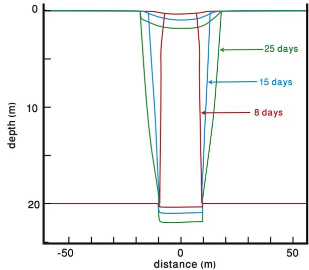
**Fig. 8.** Cavity configuration evolution for a mixed damage and visco-elastic controlled simulation of deformation caused by a 20 m-wide underlying cavity. These results are similar to field observations in the mud-flat (Fig. 2a).
