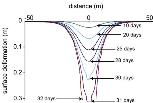
**Fig. 7.** Surface deformation evolution for a mixed damage and visco-elastic controlled simulation of deformation caused by a 10 m-wide underlying cavity. Because the surface undergoes ductile deformation prior to the collapse this sinkhole is classified as Sagging-Collapse sinkhole. These results are similar to field observations in the mud-flat (Fig. 2a).
