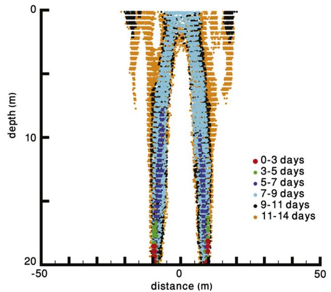
**Fig. 5.** Micro-seismic events for a damage simulation of deformation triggered by a 20 m-wide underlying cavity. These results are similar to field observation in the alluvial fans (Fig. 2b).
