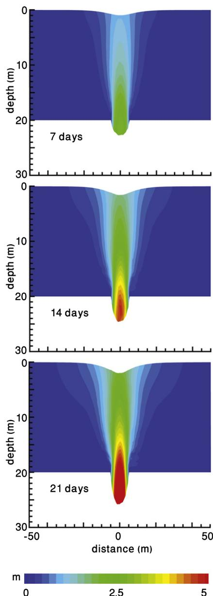
Fig. 3. Absolute displacements for a visco-elastic simulation of deformation caused by a 10 m-wide underlying cavity. No steep walls are created in this process.
