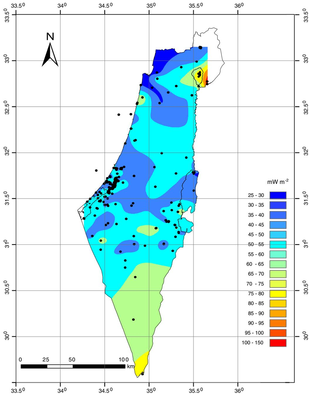
**Fig. 4.** Calculated geothermal heat flux in Israel from borehole temperature measurements. South east of the Sea of Galilee and in southern Israel the heat flux is relatively high. Black dots represent the boreholes used for the calculation and interpolation.
