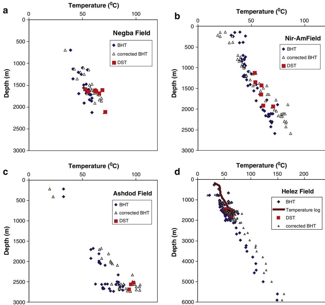
**Fig. 3.** Measured and corrected bottom-hole temperature (BHT) along with measured drill stem temperature (DST) and temperature logs. a. Negba, b. Nir-Am, c. Ashdod, and d. Helez fields (see Fig. 2 for location).
