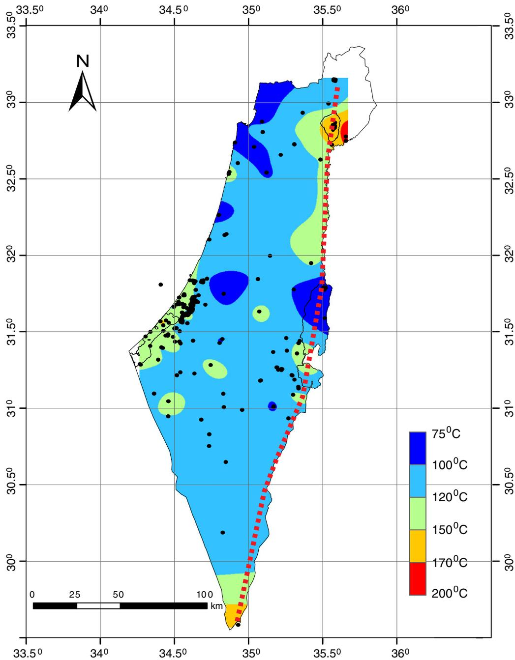
**Fig. 5.** Temperature distribution at 4 km depth. Black dots represent the boreholes used for the calculation and interpolation. The red dotted line represents the location of the cross-section showed in Fig. 6.
