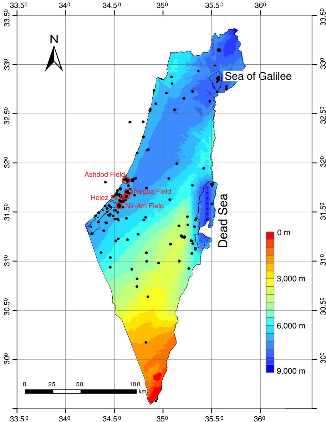
**Fig. 2.** The depth of the crystalline basement from the surface (after Rybakov and Segev, 2004; Segev et al., 2006). This depth represents the sediment thickness. In southern Israel the basement is exposed. The boreholes from which data was taken are marked by black dots.
